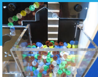
Cap hopper holds up to 1,000 2 ml cryovials (dependent on cap size)
