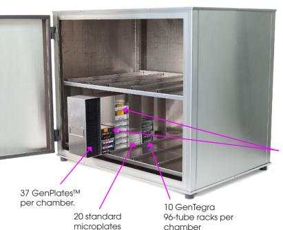
Using laboratory standard carriers make storing mixed sample carriers convenient and easy.
